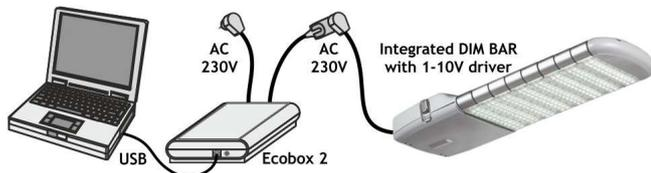
The DIM BAR programming can be done by using the Ecostream 2 software and the powerline master controller Ecobox 2 which is connected to a PC via USB connection. Ecobox 2 modulates encoded instructions into the supplying mains.
