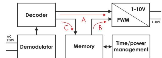
The DIM BAR does not contain a real-time clock, it has an interval counter.
