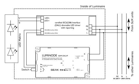
Setting the control intensity levels according to DIN input switching (motion sensor)
