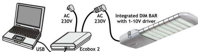
The DIM BAR programming can be done by using the Ecostreet 2 software and the powerline master controller Ecobox 2 which is connected to a PC via USB connection. Ecobox 2 modulates encoded instructions into the supplying mains. The DIM BAR then demodulates the signal, performs the decoded instruction and stores the dimming sequence into its memory. A successful programming will be indicated by fluctuating amplitude between 1V a 10V with a period of 1 second.
