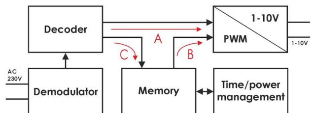
The DIM BAR does not contain a real-time clock, it has an interval counter.
