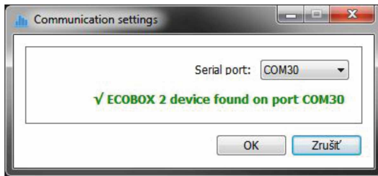
Pic. 1 Ecobox II connected to PC on port COM
