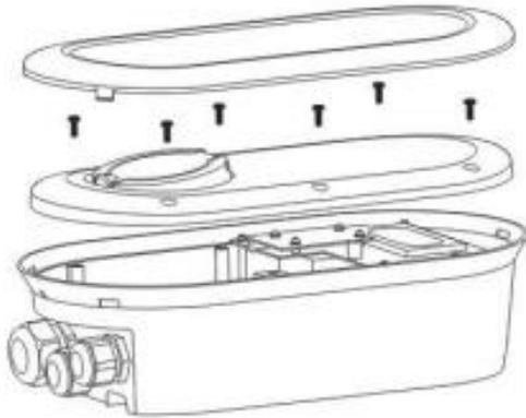
Fix the device on the wall by inserting the screws and waterproof gaskets.
