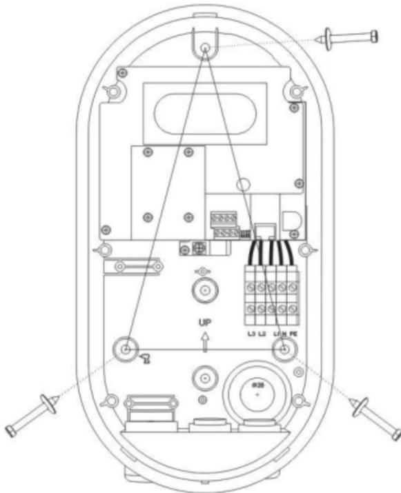
Connect the wires according to the following picture:
